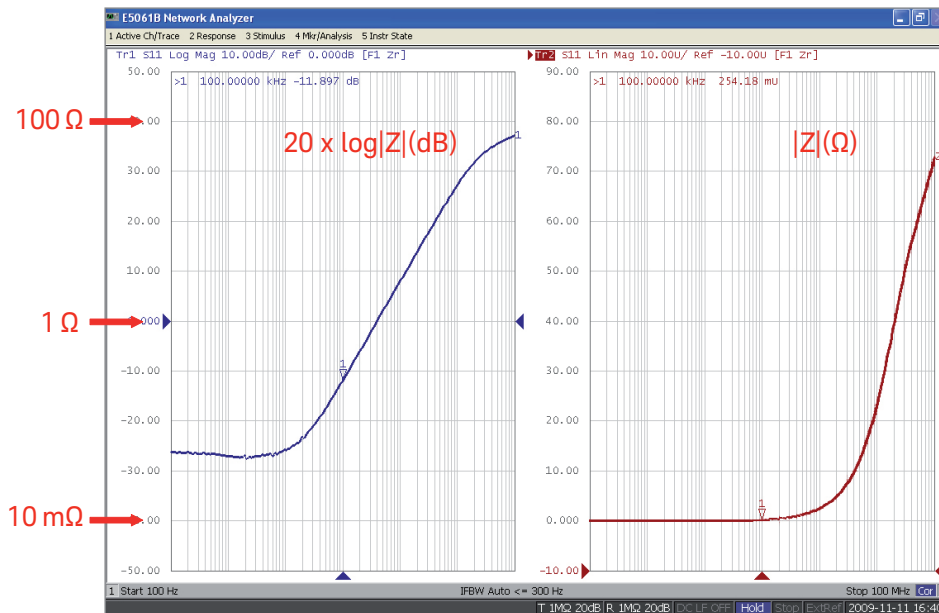
Figure 38. Output impedance measurement example
